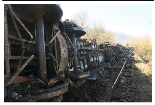
Figure 3.1.3: Appearance of the derailed wagons
