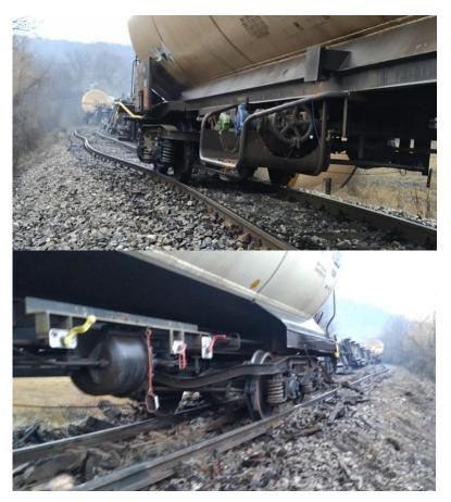
Figure 3.1.4: Appearance of the derailed ninth (up) and fourteen wagon (down) (source: "IŽS"a.d.)
