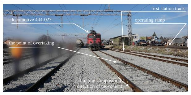
**Figure 4.1.1.1:** The appearance of the serious accident after the overtaking of the shunting composition on the railway worker (view from direction of the switch block 2 to the station facility)
