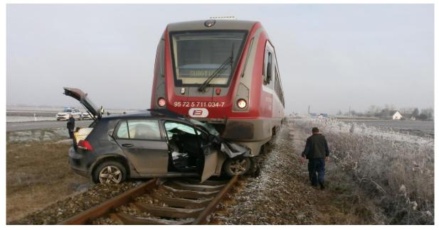
**Figure 3.4.2:** Appearance of the road passenger vehicle after the serious accident (view from the railway line, in the direction opposite from the direction of train movement, source: "IŽS"a.d.)
