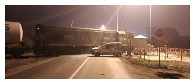
**Figure 3.1.1:** Appearance of the shunting locomotive 661-155 and the road passenger vehicle after the serious accident (view from the road, in the direction opposite to the direction of the road passenger vehicle movement, source: "NIS"a.d.)
