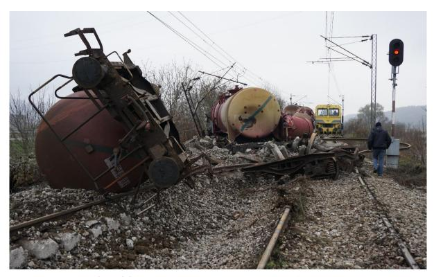
Figure 3.3.1: The view of the accident site (the point of derailment)
